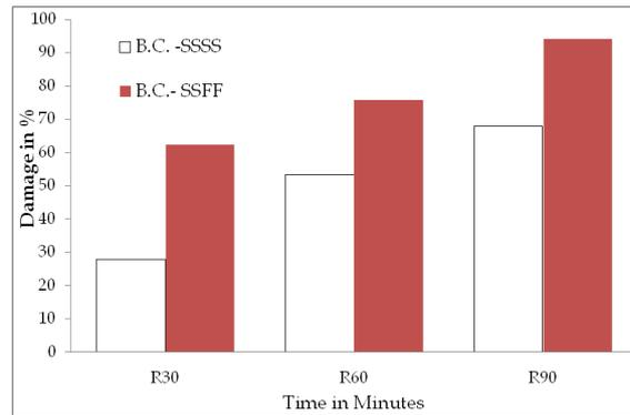
**Figure 11: Percentage of Damage versus Time for Various Boundary Conditions of Concrete Slabs**
