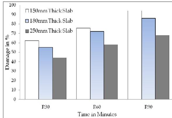
**Figure 9: Percentage of Damage versus Time for Various Thicknesses of Concrete Slabs**
