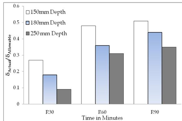
**Figure 7: Comparison of Finite Element Slab Deflection with BS 476 Code Provision, Subjected to Dead Load Only**
