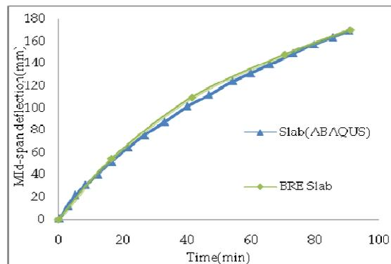
**Figure 1: Comparison of ABAQUS Model with Experimental Results of Gordon M. E. Cook [13]**
