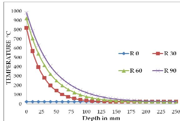
Figure 4: Variation of Temperature for 250mm Thick Slab
