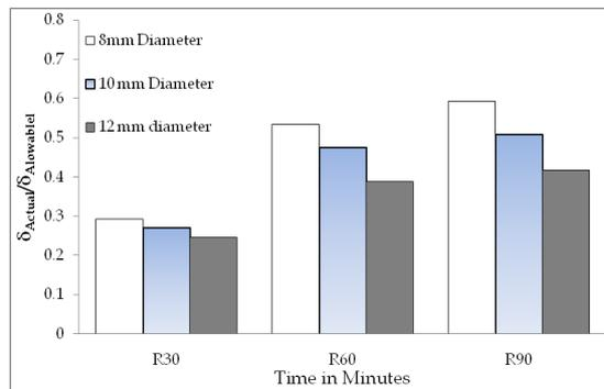
**Figure 5: Comparison of Finite Element Slab Deflection with BS 476 Code Provision, Subjected to Dead Load Only**
