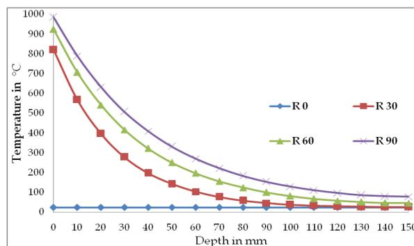
**Figure 2: Variation of Temperature for 150mm Thick Slab**
