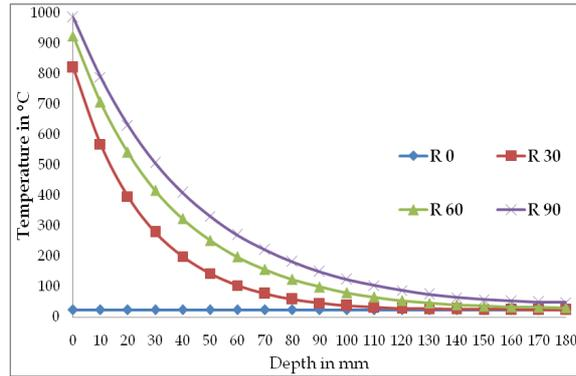
Figure 3: Variation of Temperature for 180mm Thick Slab
