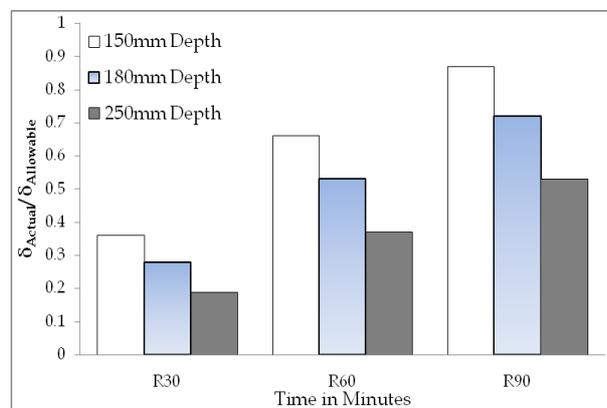
**Figure 8: Comparison of Finite Element Slab Deflection with BS 476 Code Provision, Subjected to Dead Load and Live Load**
