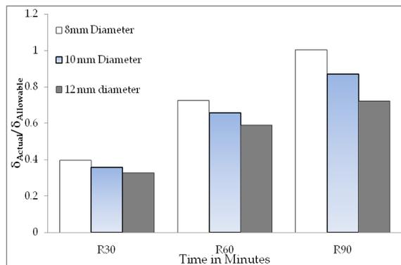
**Figure 6: Comparison of Finite Element Slab Deflection with BS 476 Code Provision, Subjected to Dead Load and Live Load**
