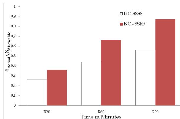
**Figure 10: Comparison of Finite Element Slab Deflection with BS 476 Code Provision**
